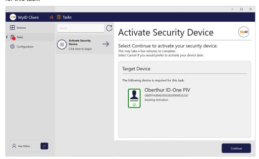
For device activation, you must use a specific device; the MyID Client for Windows displays the device type and serial number of the device you need to activate.
